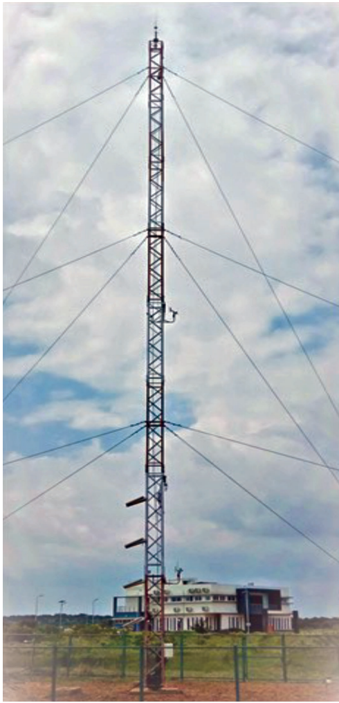
Figure-3: 32-meter meteorological tower measuring wind speed, wind direction, ambient temperature and relative humidity at 5 different levels.
