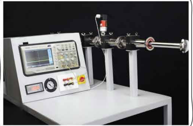
The Reddy Tube, a shock tube developed by Super-Wave Technologies
