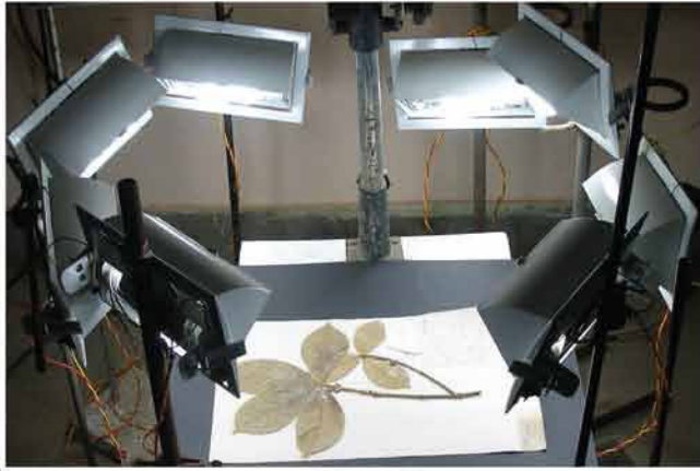
A device to scan a herbarium sheet. The image will be fed to a digital database of plants
