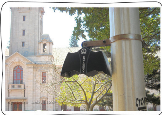
The Envirobat air quality monitoring device being field tested on the IISc campus
