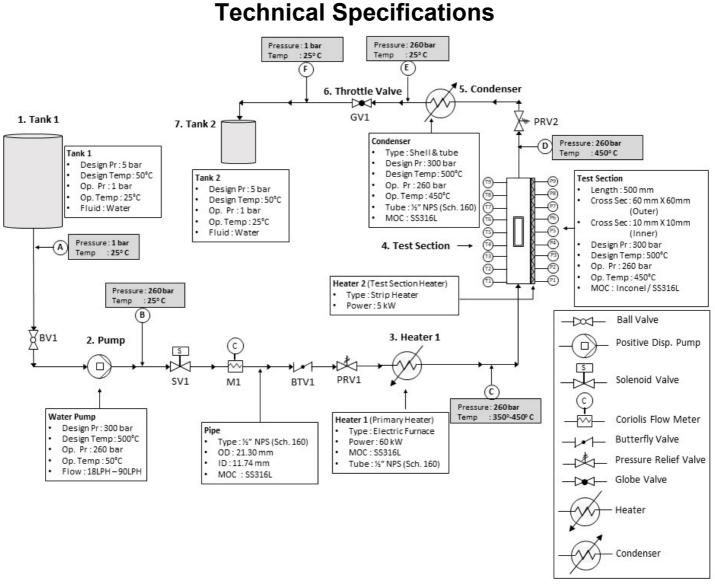
The above shown figure is the piping and instrumentation diagram (P&ID) of the supercritical steam based open loop. The conditions mentioned in the P&ID correspond to primary experimental conditions, however general range of operating conditions at various points in the loop are given below.
