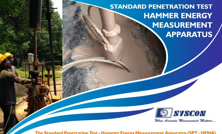
The Standard Penetration Test - Hammer Energy Measurement Apparatus (SPT - HEMA) is a Measurement Apparatus consisting of instrumented rods incorporated with force, acceleration sensors and Data recording cum Processing unit. It measures the Energy Transferred by SPT Hammers below Anvil and above Split Spoon sampler.
