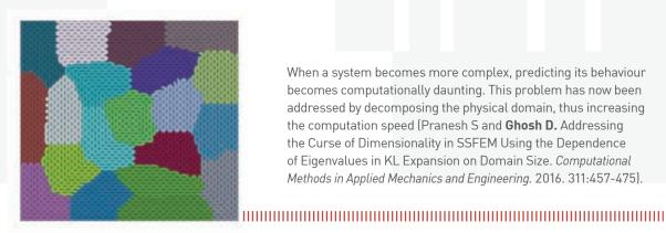
When a system becomes more complex, predicting its behaviour becomes computationally daunting. This problem has now been addressed by decomposing the physical domain, thus increasing the computation speed (Pranesh S and Ghosh D. Addressing the Curse of Dimensionality in SSFEM Using the Dependence of Eigenvalues in KL Expansion on Domain Size. Computational Methods in Applied Mechanics and Engineering. 2016. 311:457-475).
