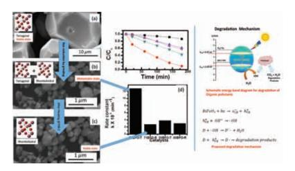
used as photocatalysts for degradation of a typical organic pollutants, Rhodamine B. We found that the degradation rate increased five times when the catalysts were in the metastable state (d) (Narayan B, Adhikari S, Madras G and **Ranjan R.** Trapping a Metastable Ferroelectric Phase by Size Reduction in Semiconducting Ferroelectric BiFeO $_3$ -PbTiO $_3$  and its Implications for Photocatalytic Response. *Physical Review Applied*. 2017. 7:024018).
