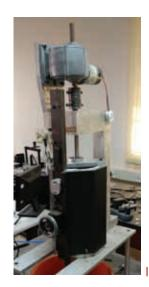
The Couette Cell and apparatus to conduct experiments to understand vortex flow in sheared granular materials (Krishnaraj KP and Nott PR. A Dilation-Driven Vortex Flow in Sheared Granular Materials Explains a Rheometric Anomaly. Nature Communications. 2016. 7:10630).
