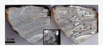
Spheroidal weathering of a diabase in hand-specimen scale. (Banerjee A, Chakrabarti R and Mandal S. Geochemical Anatomy of a Spheroidally Weathered Diabase. Chemical Geology. 2016. 440:124-138).
