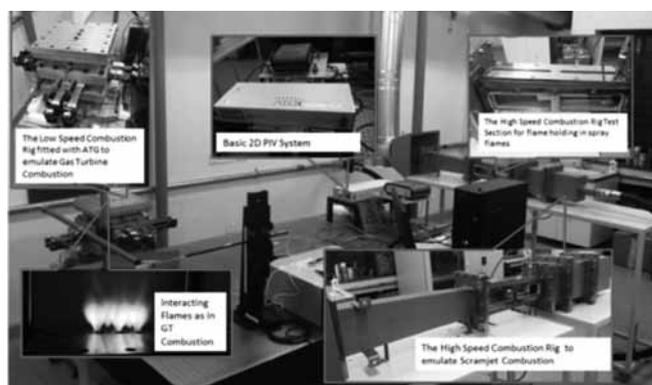
**Figure 2:** New facilities in the turbulent combustion and spray research laboratory
