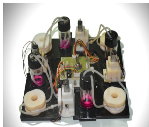
Perfusion bioreactor that can accommodate scaffolds on cover-slips with provision for high magnification in situ
