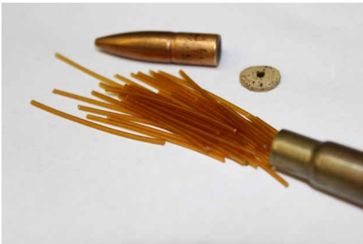
Cordite filaments manufactured in 1964 in a .303 British Rifle cartridge
