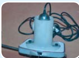
Micro N, a micro newton force sensor
