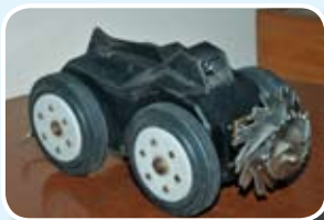
Scorpionok, the sewer cleaning robot
