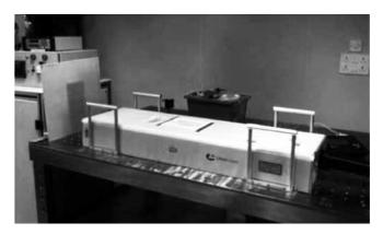
**Figure 1:** Nd-YAG LASER: R850mJ @ 1064 nm; Beam Dia: 9.5mm, pulse6-9 nsec; Reptn Rate 10 Hz
