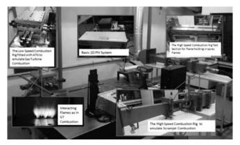
Figure 2: New facilities in the turbulent combustion and spray research laboratory
