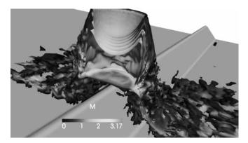
**Figure 4:** Supersonic round jet impinging on wedge from a Large Eddy Simulation. Density iso-surfaces coloured by Mach number
