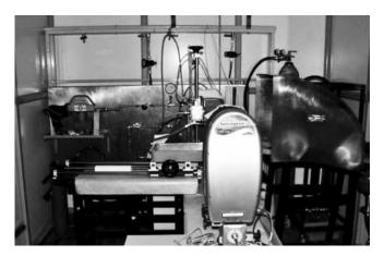
Figure 3: Spray drop size measurement system (Spraytec from Mavern Instruments, UK)
