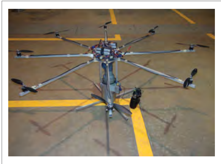
A drone with a nanomist generator for pesticide and nutrient delivery
