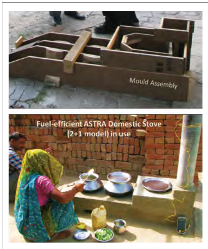
A mould for rapid construction of fuel efficient ASTRA domestic stove
